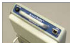
Ethernet communications 100Mbit/s
